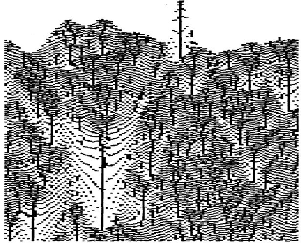
FIG. 4. Growing aggregate of ballistic-deposition model with partial sliding for power-law noise of \mu = 2 and L = 150 .
